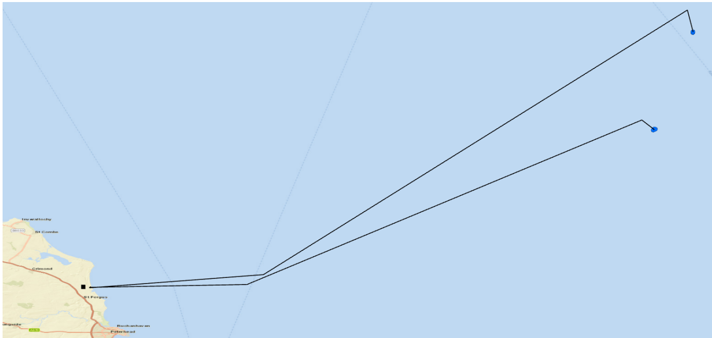
Figure 46- Cable connections from Buzzard or Golden Eagle shown on GIS
