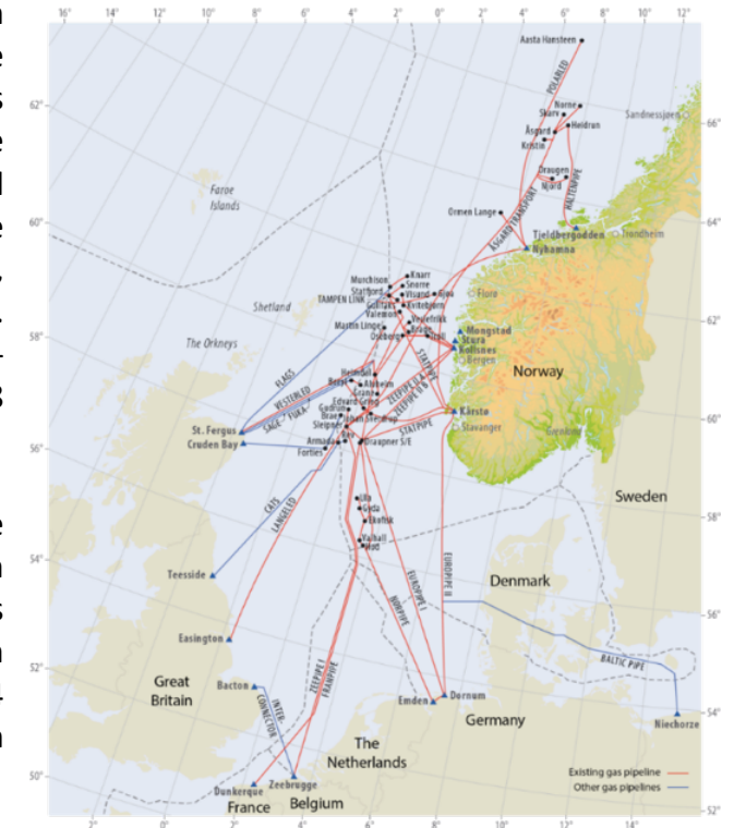
Figure 65- Existing gas pipeline in the Norwegian continental shelf (Norwegian Petroleum, 2024)
