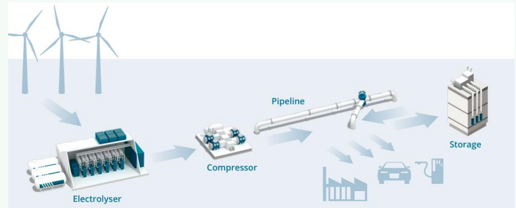
Figure 60- simplified version of an onshore hydrogen production station (Peter Adam et al., 2020)
